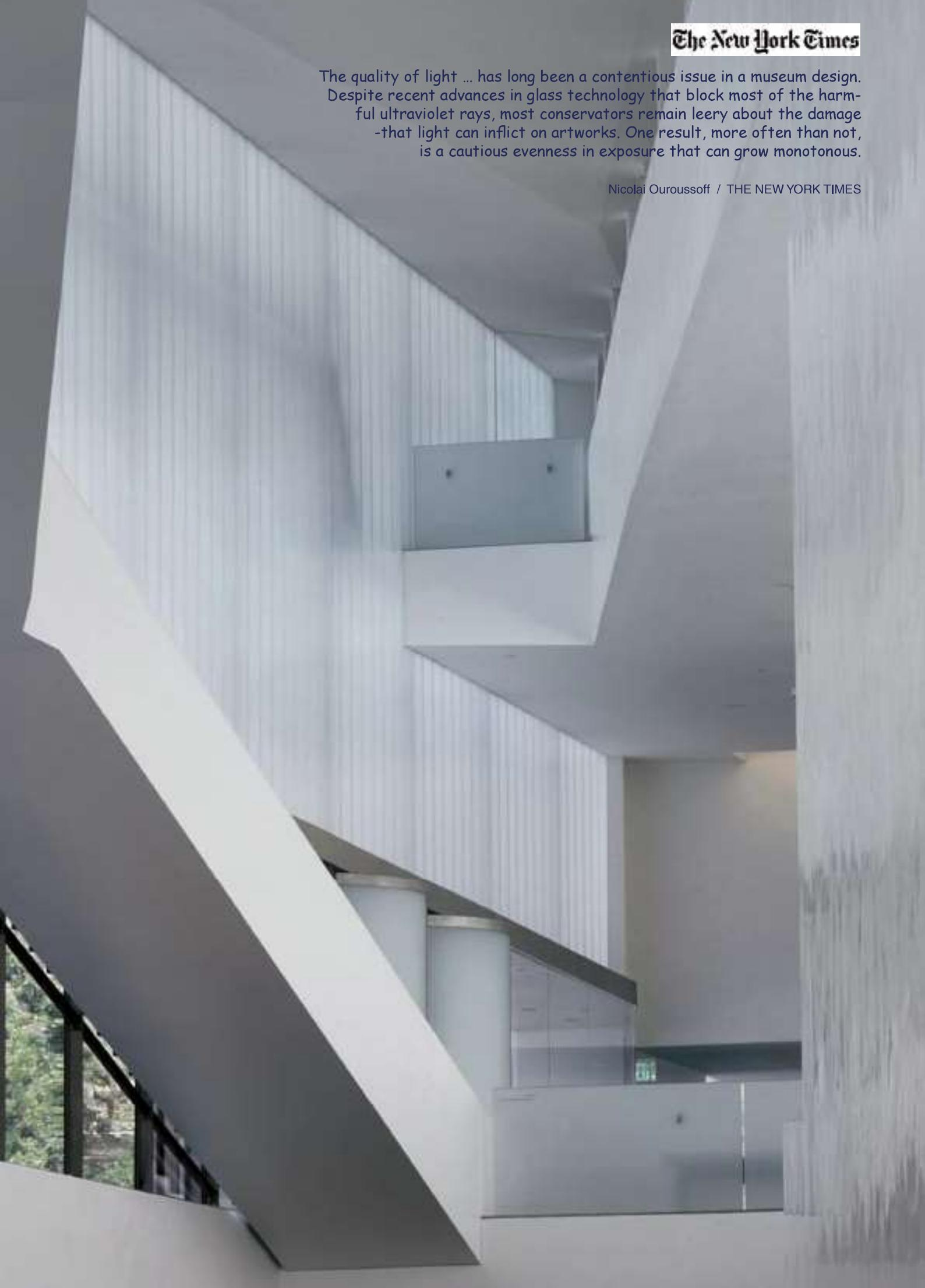
Mr. Holl solves the problem by varying the height of his galleries from 27 to 34 feet. This allows for architectural spaces enlivened by shifting natural light. Big, curved panels inside the lenses funnel a mix of northern and southern sunlight down into the galleries, so that you are aware of the passing of a cloud or a bit of thunder.
